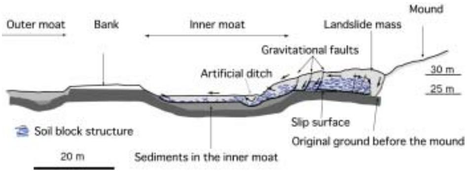
Fig.5. Cross-section of the landslide along the trench in 2000.
