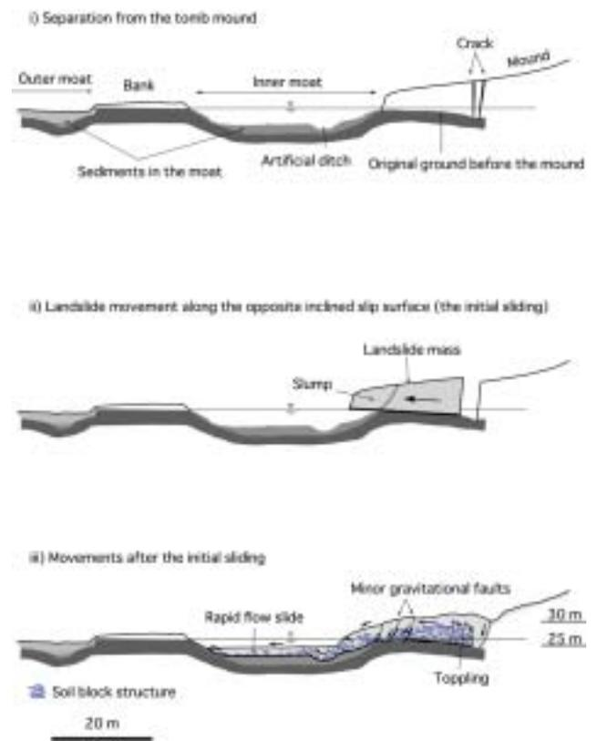
Fig.7. Process of collapse within the landslide.
