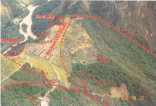
Fig. 7 Oblique airphoto of the Inca citadel, indicating delineation of existing and potential landslides.
