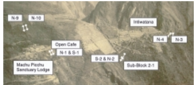
Fig. 9 Location of extensometers in the Front Slope of Machu Picchu citadel.
