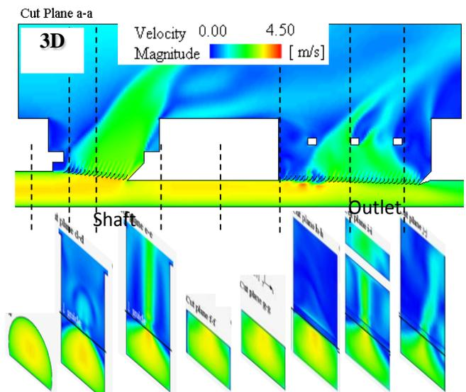
A distribution of vehicle gases in a target tunnel
