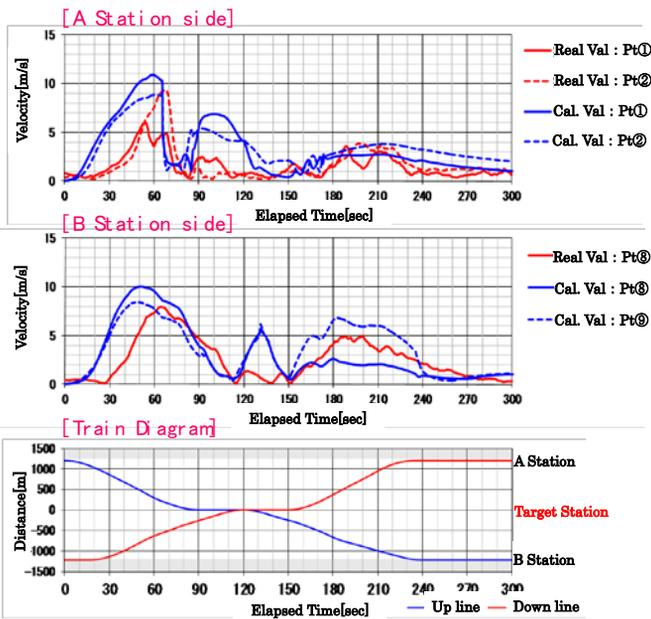
Time-changes in train winds (comparison between simulated and observed wind velocities)
