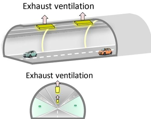
An image of the structures ventilating vehicle gases in a road tunnel
