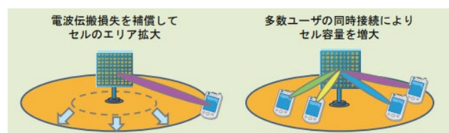
図-7 Massive MIMOの導入効果 4)
