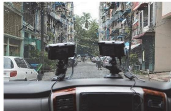
Photo 5 Two Cameras Setting in a Car Dashboard
