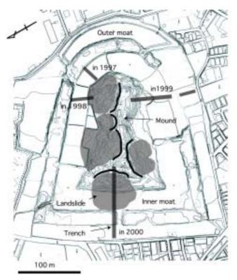
Fig.2. Plan view and landslide distribution in the Imashirozuka mound.
