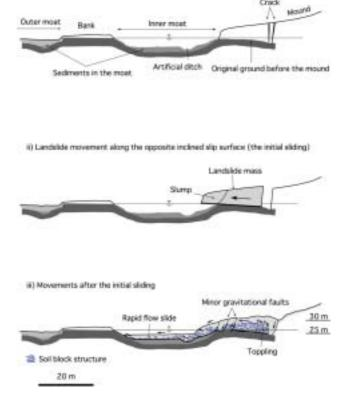
Fig.7. Process of collapse within the landslide.
