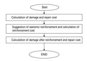
Fig. 8 Flow to acquire damage and cost.
