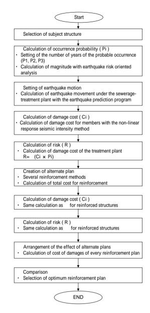
Fig. 1. Flow of selection for aseismic reinforcement method.
