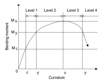
Fig. 4 Damage level concept.
