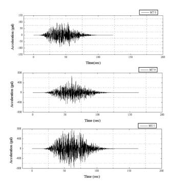
Fig.7 Waveforms of earthquake motion L1, L2, and L3
